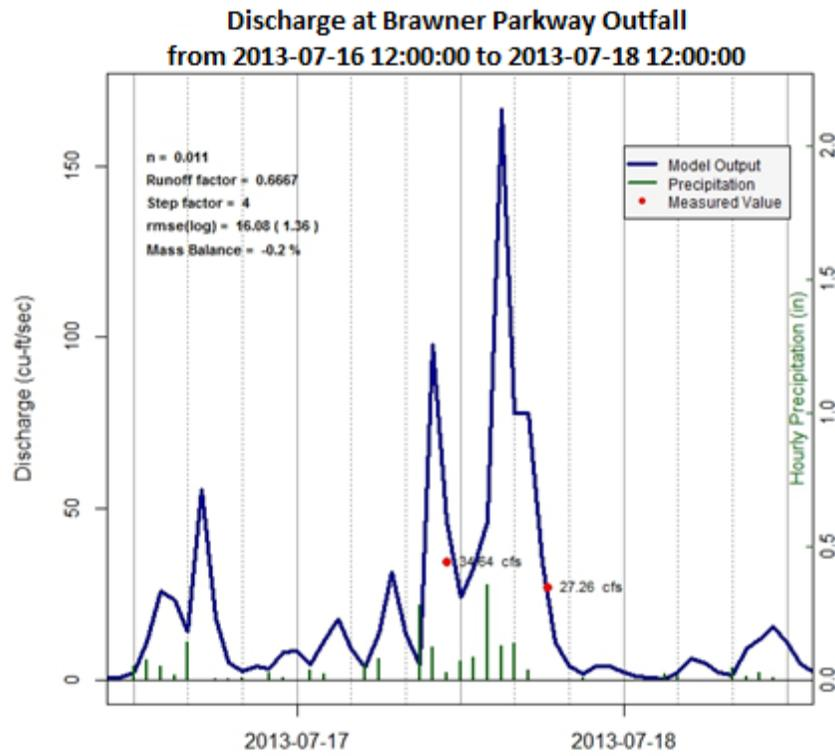
Figure A.1. Modeled discharge, precipitation, and calibration points at Brawner Parkway Outfall near Ropes Park on June 30, 2013 and July 17, 2013
