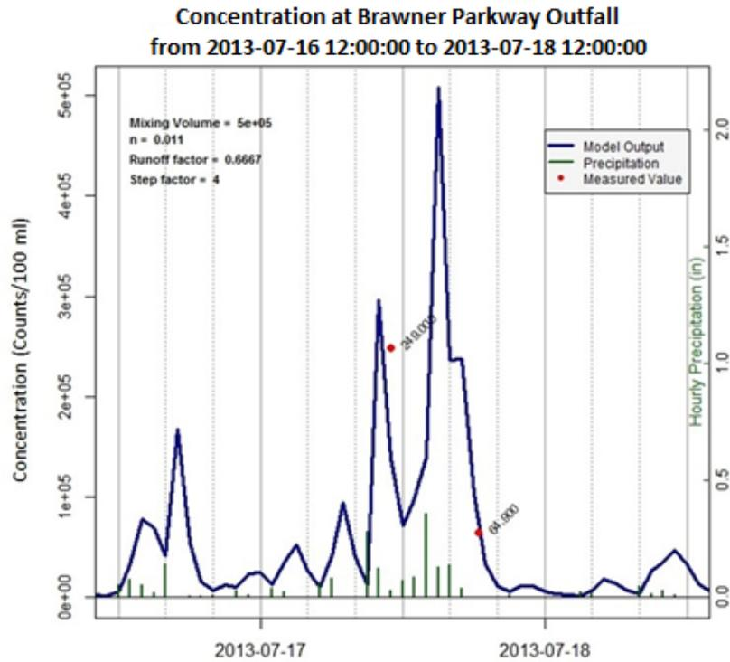
Figure A.2. Modeled bacteria concentrations, precipitation, and calibration points at Brawner Parkway Outfall near Ropes Park on June 30, 2013 and July 17, 2013
