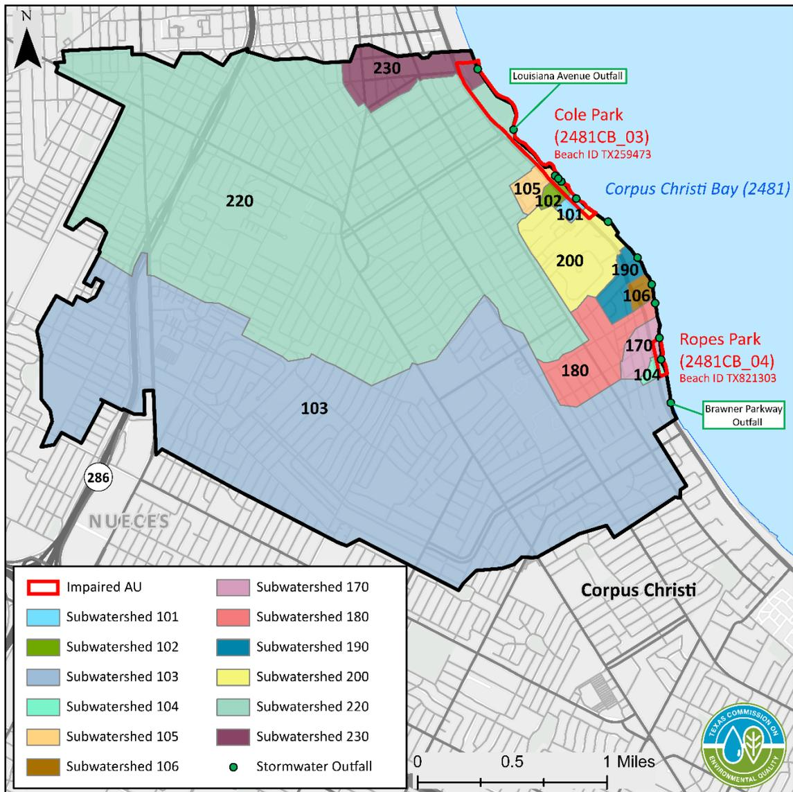
**Figure 3. TMDL watershed divided into 12 subwatersheds**
