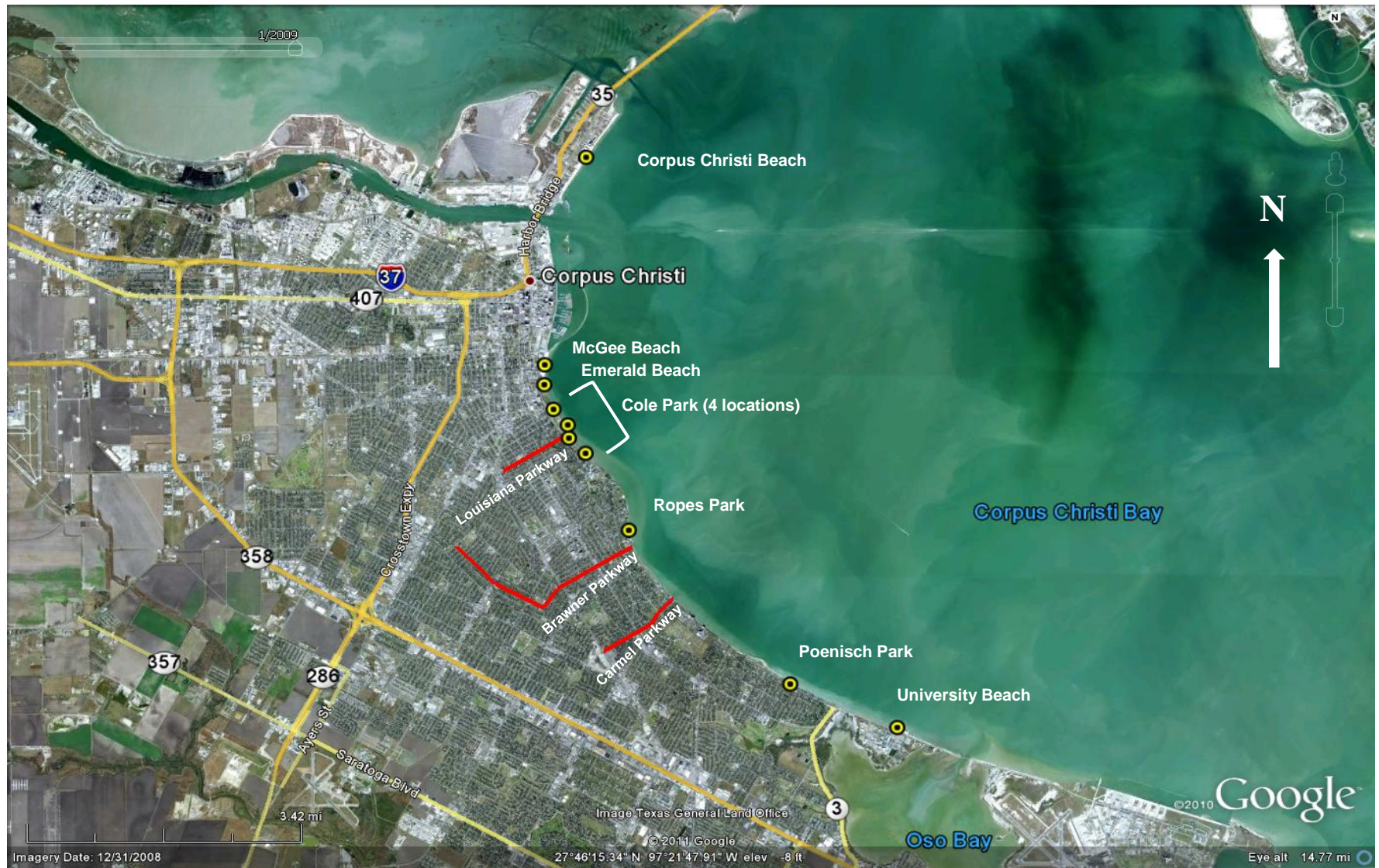
Fig. 3.1. Aerial photo depicting Corpus Christi Bay Beaches TMDL sampling locations and three major drainage ditches at Louisiana Parkway, Brawner Parkway, and Carmel Parkway. Retrieved on 4/5/2011 from Google Earth.
