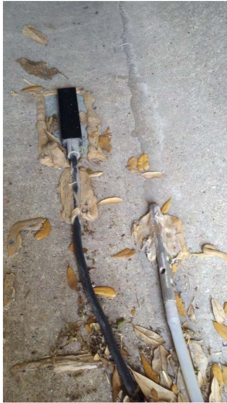
Figure 8. Sampler Tube Intake and Area Velocity Probe at Pon Court Basin Inlet.
