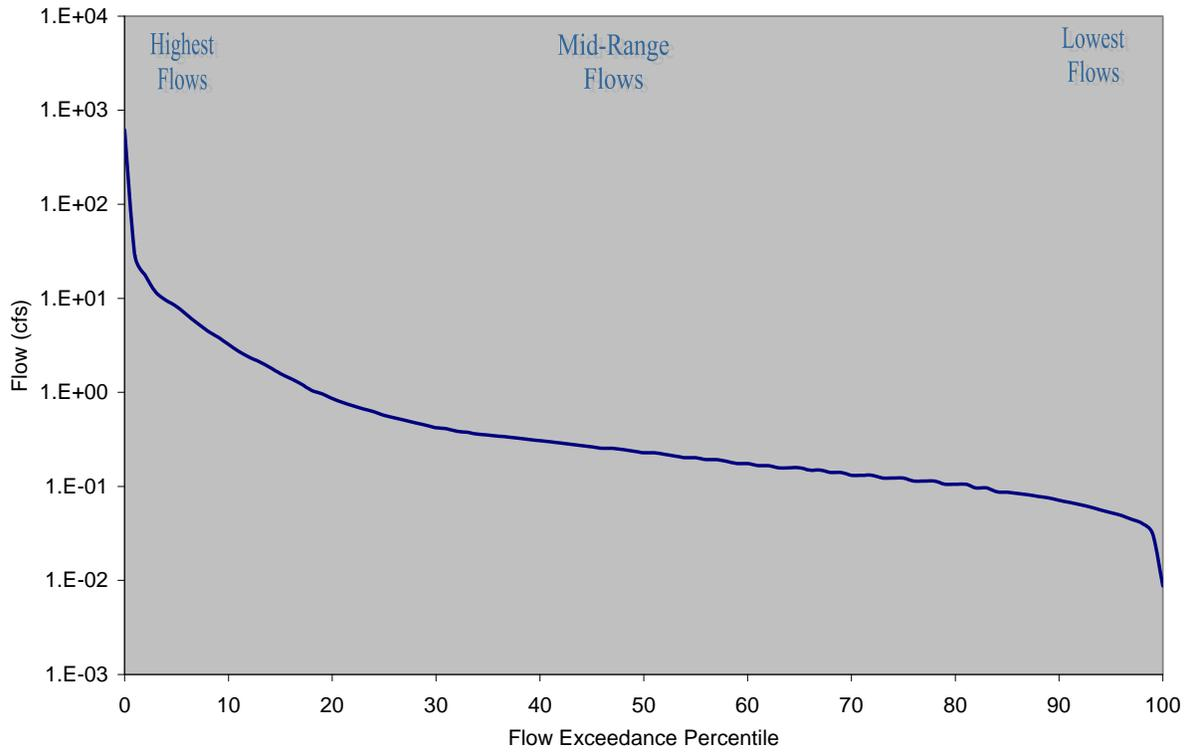
**Figure 4-5 Flow Duration Curve for Pine Gully Above Tidal (1007H\_01)**
