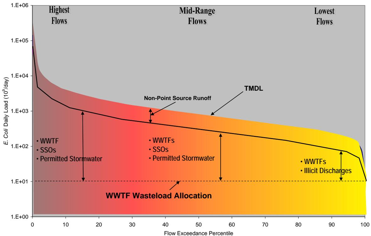
**Figure 4-12 LDC Schematic Diagram – Interpreting Sources and Loads**
