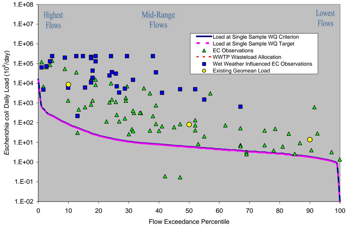
**Figure 4-18 Load Duration Curve for Plum Creek Above Tidal (1007I\_01)**
