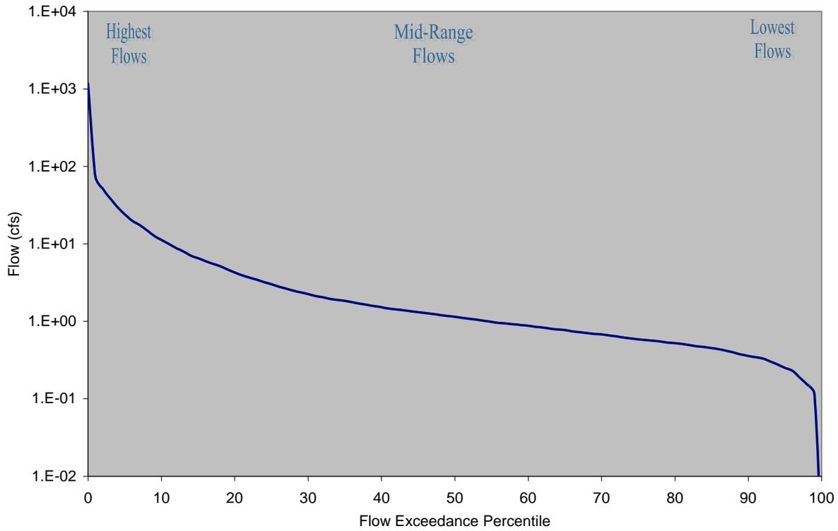
**Figure 4-2 Flow Duration Curve for Spring Gully Above Tidal (1006H\_01)**
