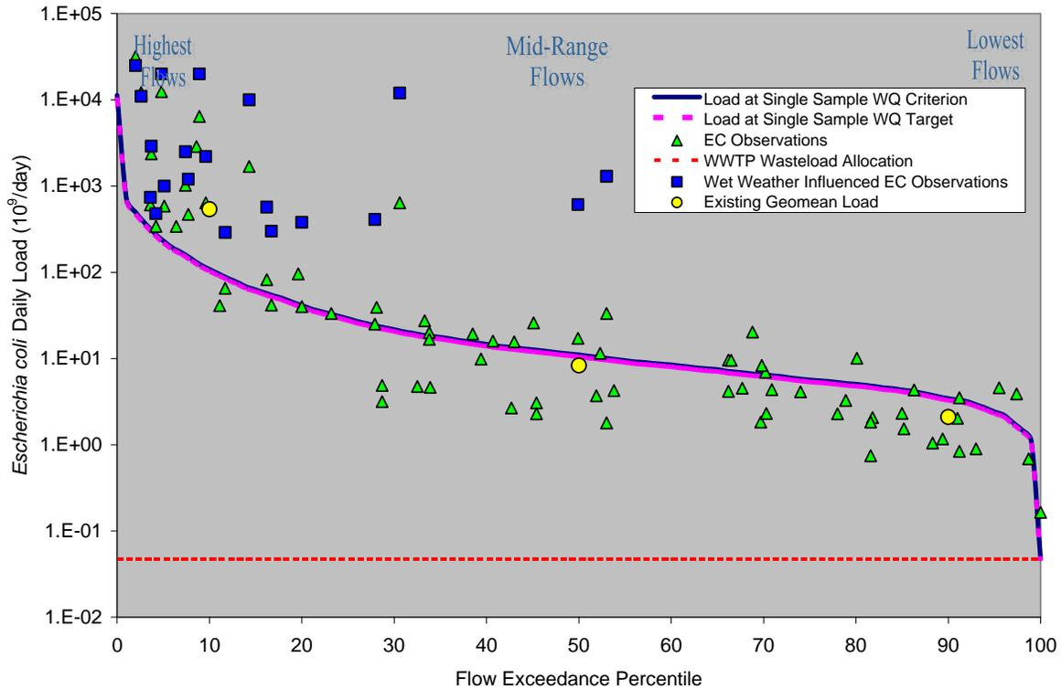
**Figure 4-14 Load Duration Curve for Spring Gully Above Tidal (1006H\_01)**
