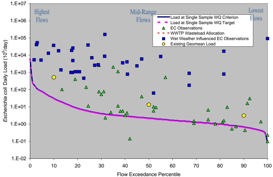
**Figure 4-17 Load Duration Curve for Pine Gully Above Tidal (1007H\_01)**
