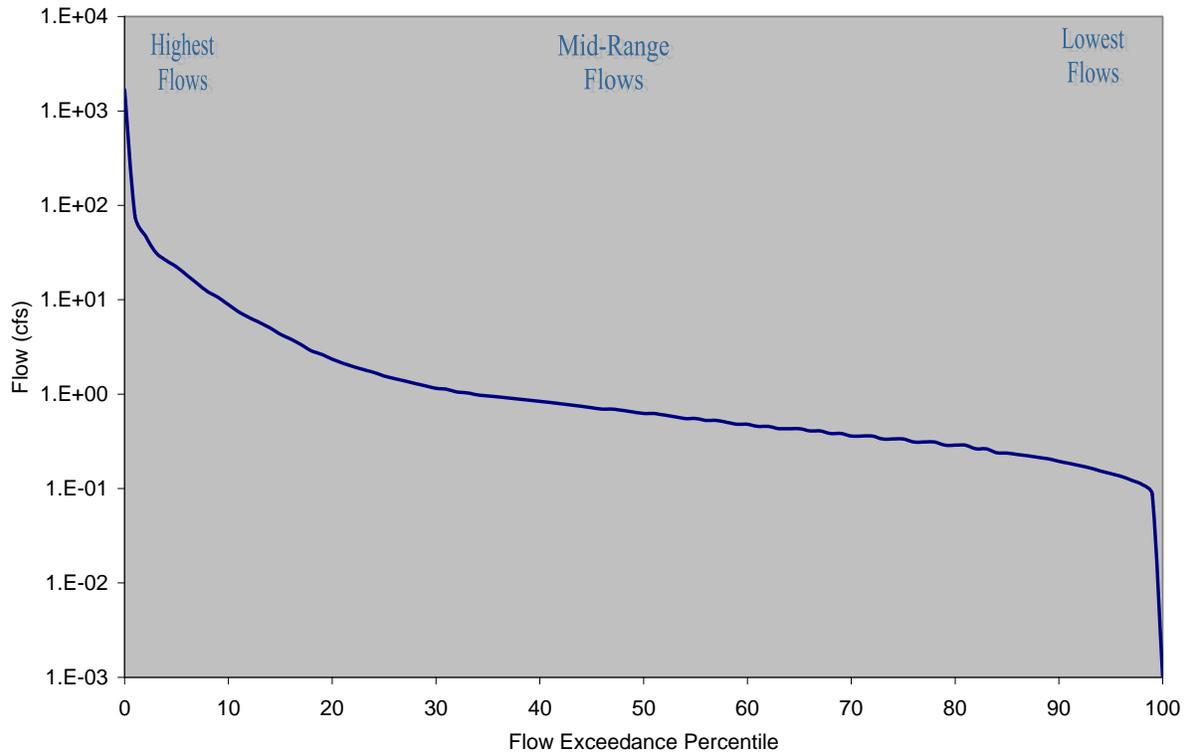
**Figure 4-6 Flow Duration Curve for Plum Creek Above Tidal (1007I\_01)**
