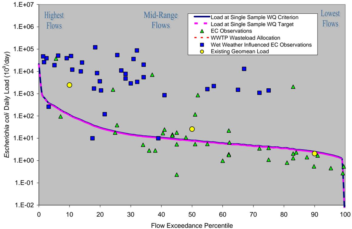
**Figure 4-16 Load Duration Curve for Kuhlman Gully Above Tidal (1007G\_01)**
