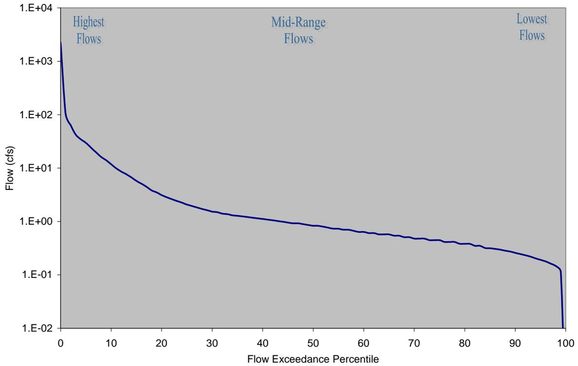
**Figure 4-4 Flow Duration Curve for Kuhlman Gully Above Tidal (1007G\_01)**
