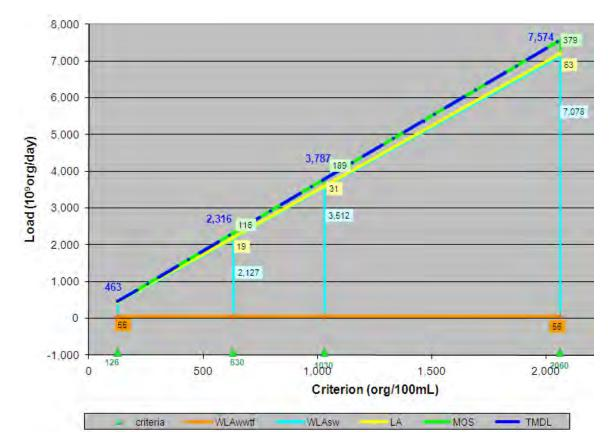
Figure A-1. Allocation Loads for AU 1006D\_01 as a function of WQ Criteria
