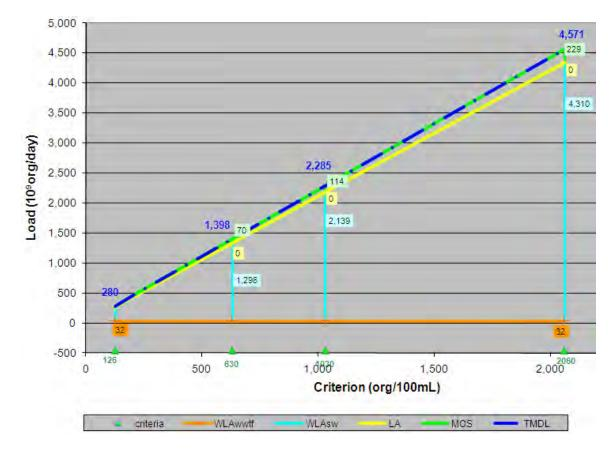
Figure A-2. Allocation Loads for AU 1006D\_02 as a function of WQ Criteria
