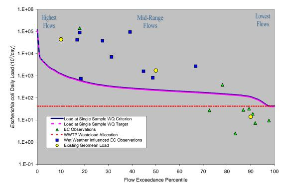
Figure 10. Load Duration Curve for *E. coli* in Halls Bayou (1006D\_01)
