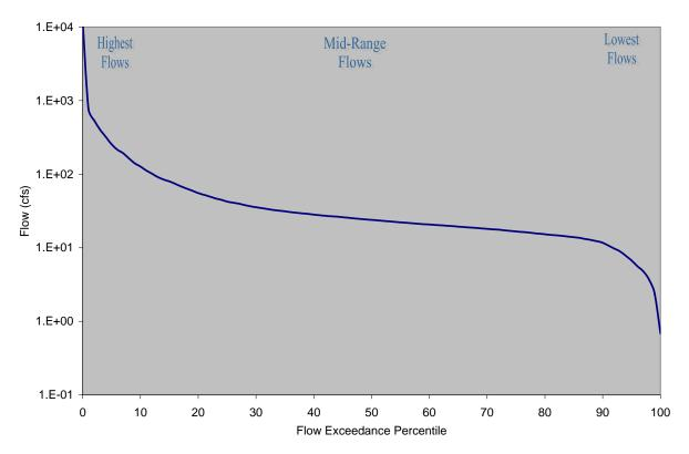
Figure 4-1 Flow Duration Curve for Halls Bayou below U.S. 59 (1006D\_01)
