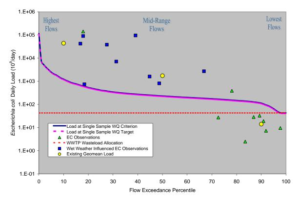
Figure 4-6 Load Duration Curve for Halls Bayou below U.S. 59 (1006D\_01)
