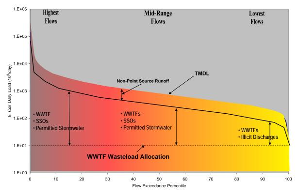
Figure 4-5 LDC Schematic Diagram – Interpreting Sources and Loads
