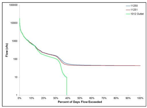
Figure13 Flow duration curve at monitoring stations on the West Fork San Jacinto River (1004\_02)
