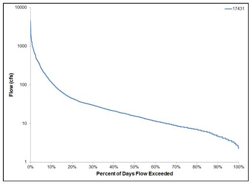
Figure 11 Flow duration curve at the monitoring station on the East Fork San Jacinto River (1003\_03)
