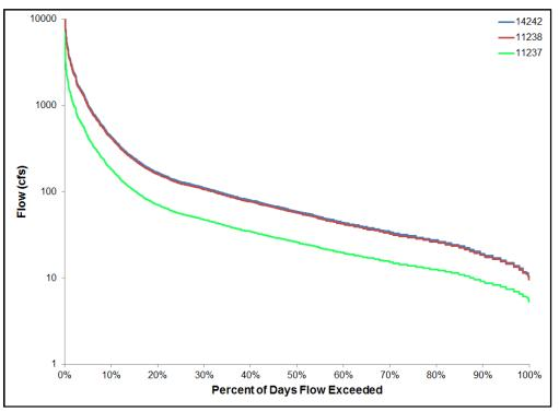
Figure 10 Flow duration curve at monitoring stations on the East Fork San Jacinto River (1003\_02)
