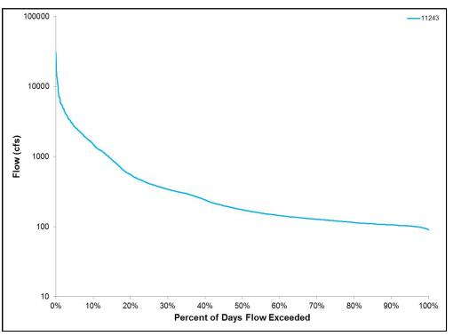
Figure 12 Flow duration curve at the monitoring station on the West Fork San Jacinto River (1004\_01)
