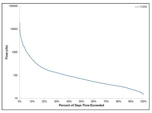
Figure 9 Flow duration curve at the monitoring station on the East Fork San Jacinto River (1003\_01)
