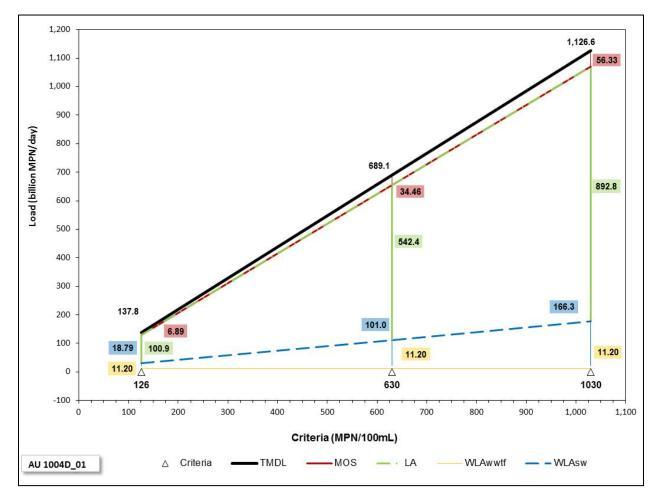
**Figure A-7.** Allocation loads for Crystal Creek (1004D\_01) as a function of water quality criteria
