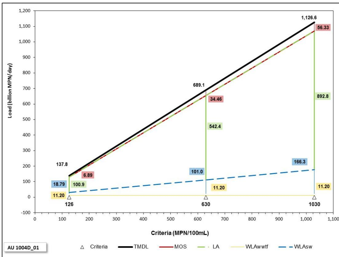
Figure A-7. Allocation loads for Crystal Creek (1004D\_01) as a function of water quality criteria
