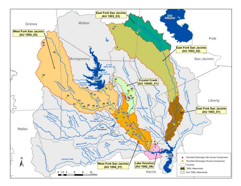
Figure 4. Permitted wastewater operations in Lake Houston, East Fork & West Fork San Jacinto rivers, and Crystal Creek TMDL watersheds
