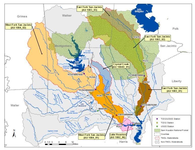
Figure 2. Lake Houston watershed showing SWQM monitoring stations and USGS gauging stations
