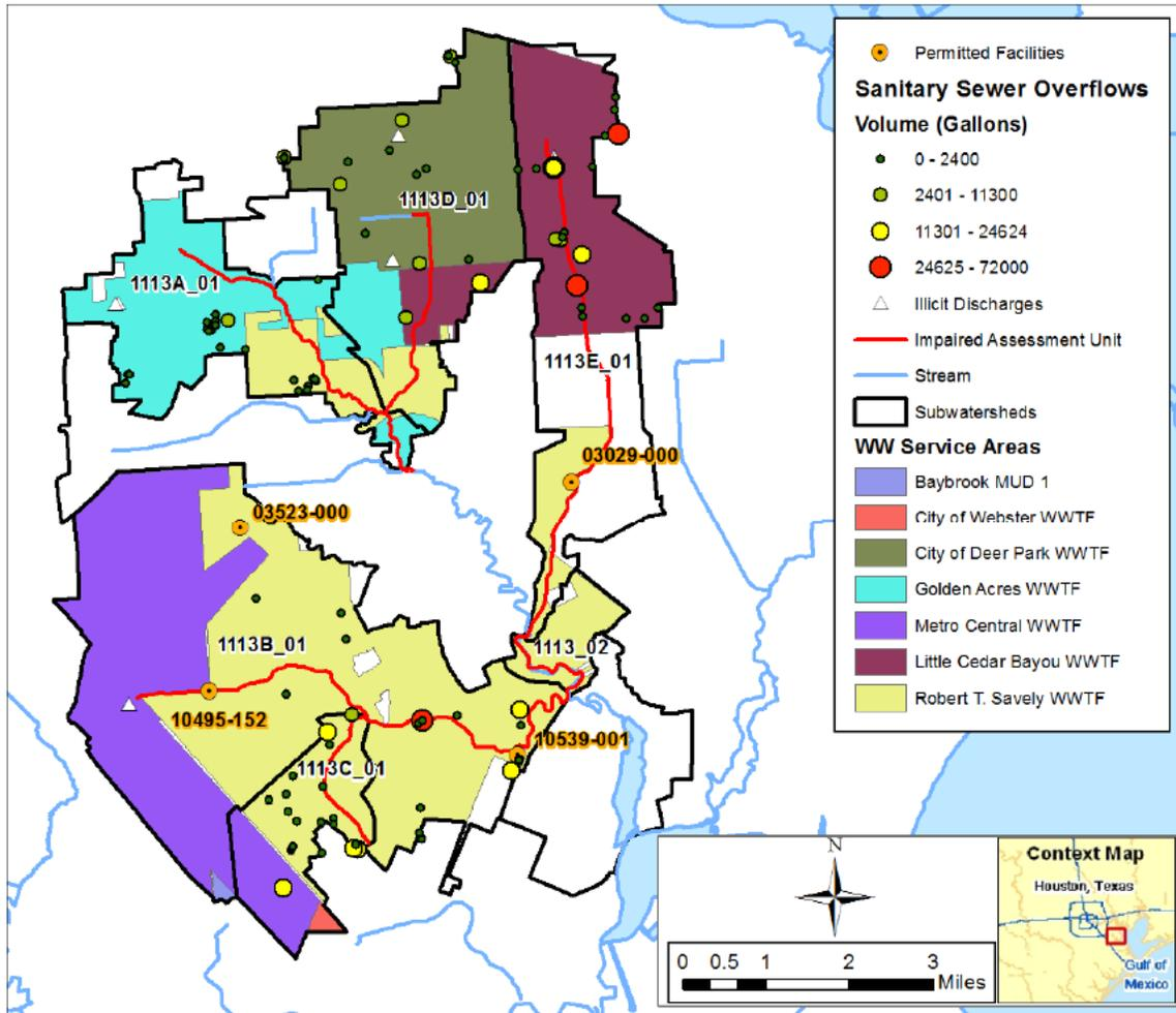
Figure 5. Sanitary Sewer Overflow Locations
