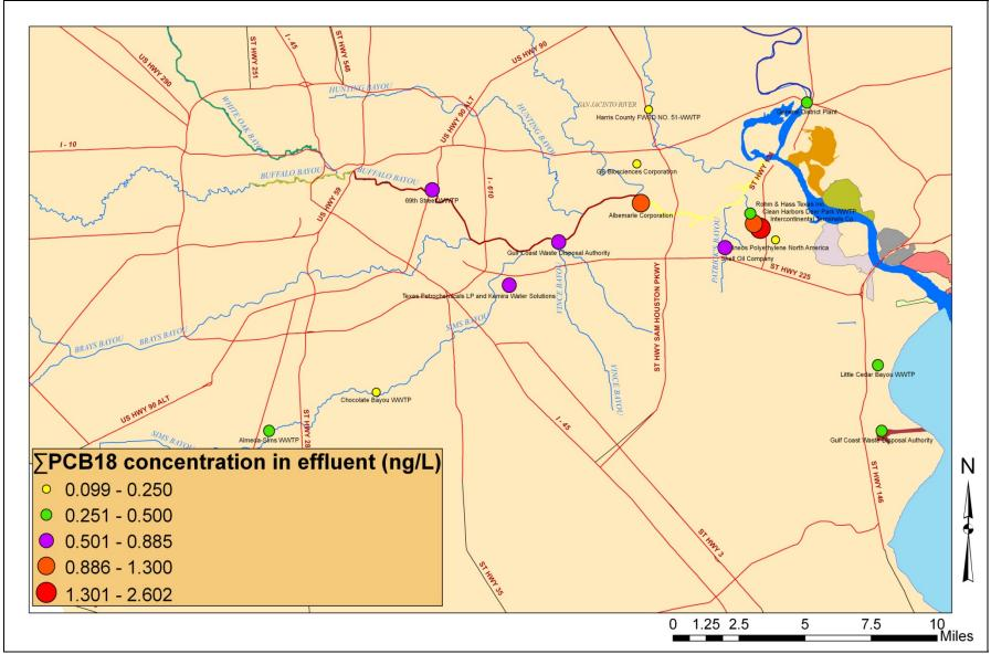
Figure 5.2c Total PCB concentrations in effluent calculated as sum of 18 congeners
