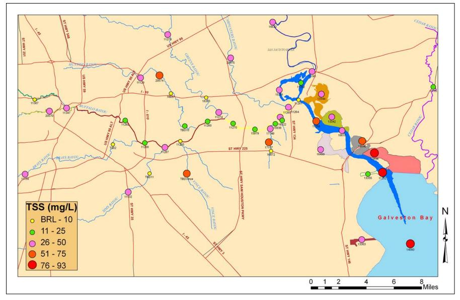
Figure 3.5 TSS measurements in water samples collected in Summer 2009
