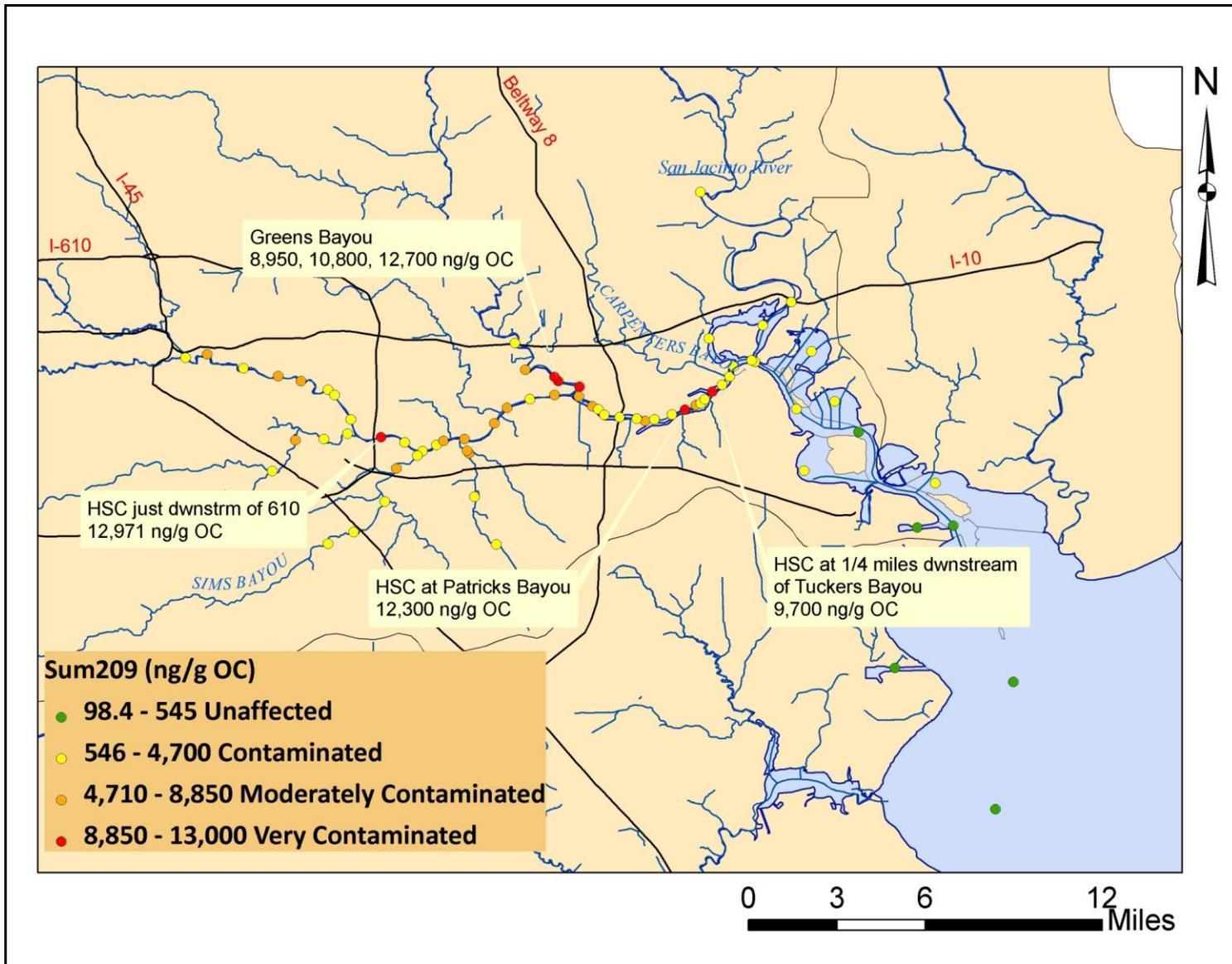
Figure 5.14 2008 sediment PCB concentration map
