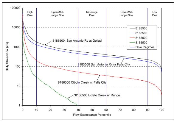
Figure 8: Flow Duration Curves for USGS Stations, Logarithmic Scale
