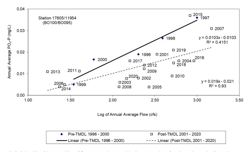
Figure 10 Relationship of the natural log of flow to annual average PO<sub>4</sub>-P concentration of routine grab samples for station 17605/11954 (BO100/BO095)
