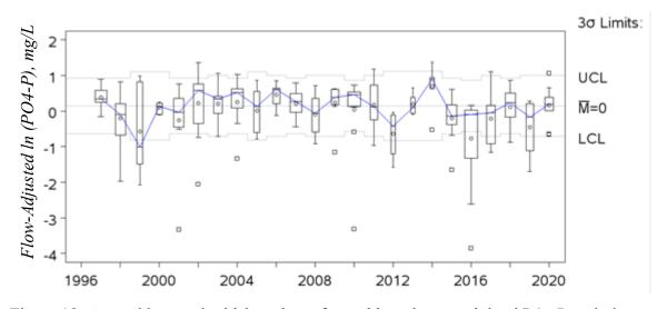
Figure 18 Annual box-and-whisker plots of monthly volume-weighted PO<sub>4</sub>-P grab data for station 17226 (BO020)
