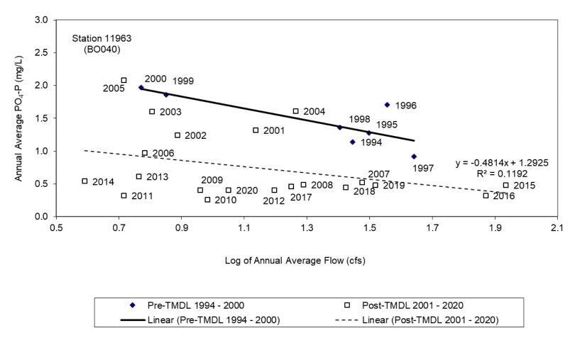
Figure 6 Relationship of the natural log of flow to annual average PO<sub>4</sub>-P concentration of routine grab samples for station 11963 (BO040)
