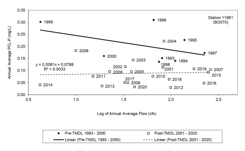
Figure 7 Relationship of the natural log of flow to annual average PO<sub>4</sub>-P concentration of routine grab samples for station 11961 (BO070)
