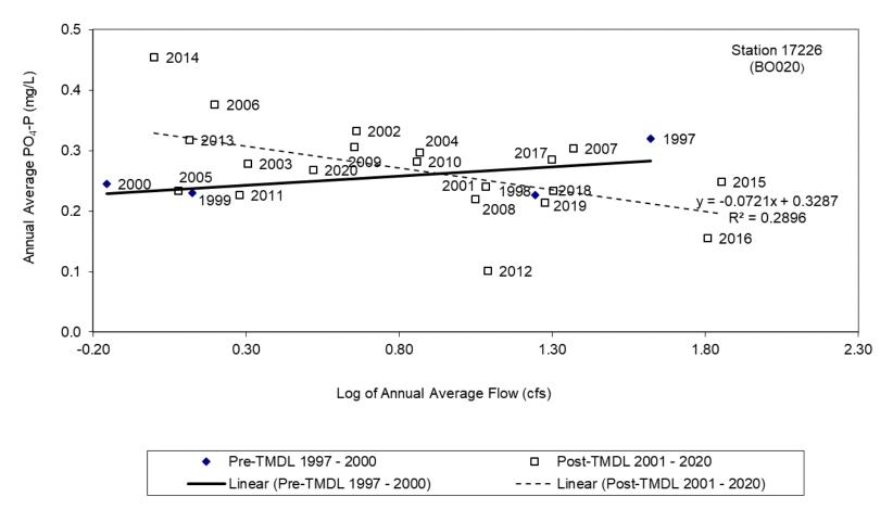
Figure 5 Relationship of the natural log of flow to annual average PO<sub>4</sub>-P concentration of routine grab samples for station 17226 (BO020)
