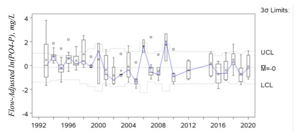
Figure 21 Annual box-and-whisker plots of monthly volume-weighted PO<sub>4</sub>-P grab data for station 13486 (GC100)
