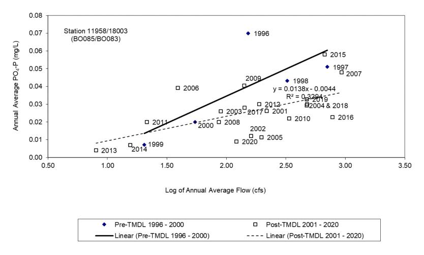
Figure 8 Relationship of the natural log of flow to annual average PO<sub>4</sub>-P concentration of routine grab samples for station 11958/18003 (BO085/BO083)
