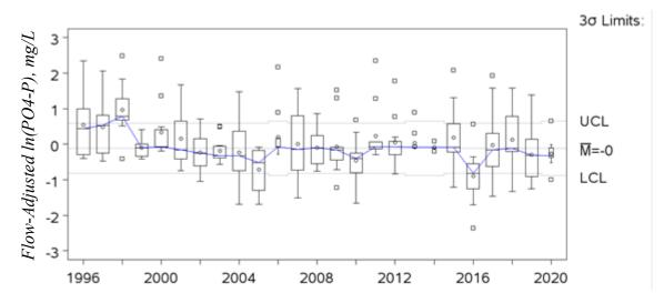
Figure 22 Annual box-and-whisker plots of monthly volume-weighted PO<sub>4</sub>-P data for station 11956 (BO090)
