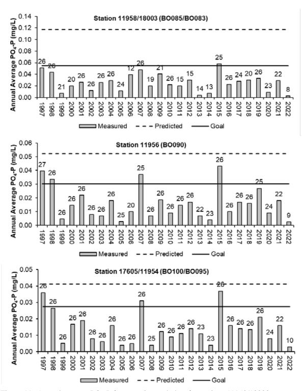
Figure 11 Annual average PO<sub>4</sub>-P from routine grab data for stations 11958/18003 (BO085/BO083), 11956 (BO090), and 17605/11954 (BO100/BO095) compared to the long-term predicted concentration without TMDL implementation and the TMDL goal
