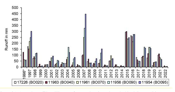
Figure 25 Annual runoff in millimeters for gaged stations along the North Bosque River
