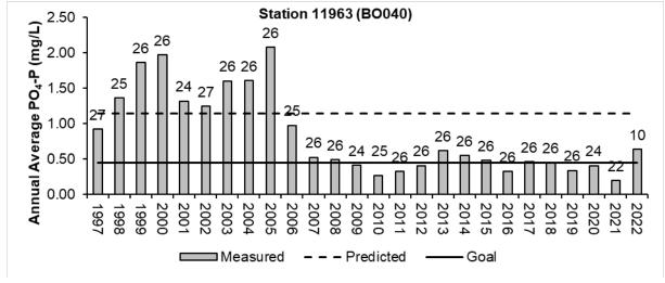
Figure 10 Annual average PO<sub>4</sub>-P from routine grab data for stations 17226 (BO020) and 11963 (BO040) compared to the long-term predicted concentration without TMDL implementation and the TMDL goal
