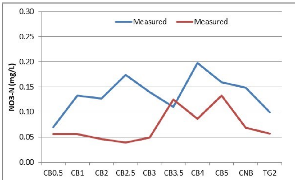
Figure H-12 Calibration of NO 3 -N in the Cow Bayou WASP model
