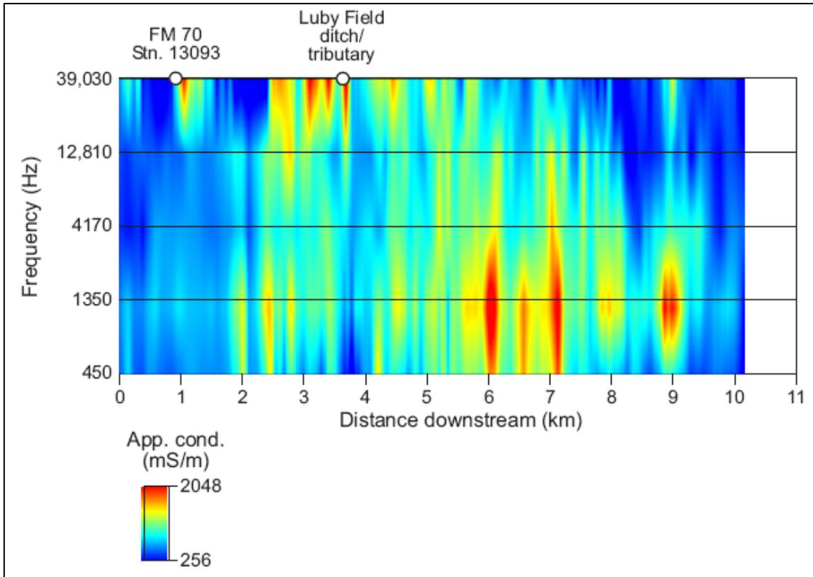
Note: The shallowest-exploring frequency is along the top of the image and the deepest-exploring frequency is along the bottom.
