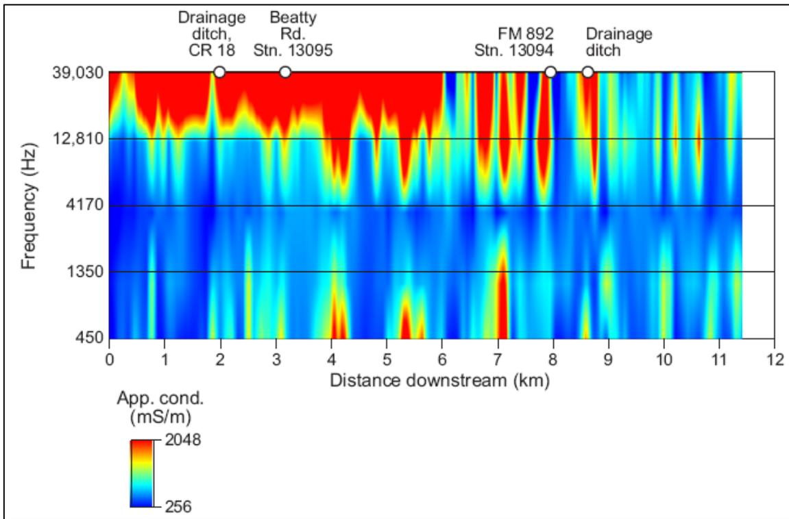
Note: The shallowest-exploring frequency is along the top of the image and the deepest-exploring frequency is along the bottom
