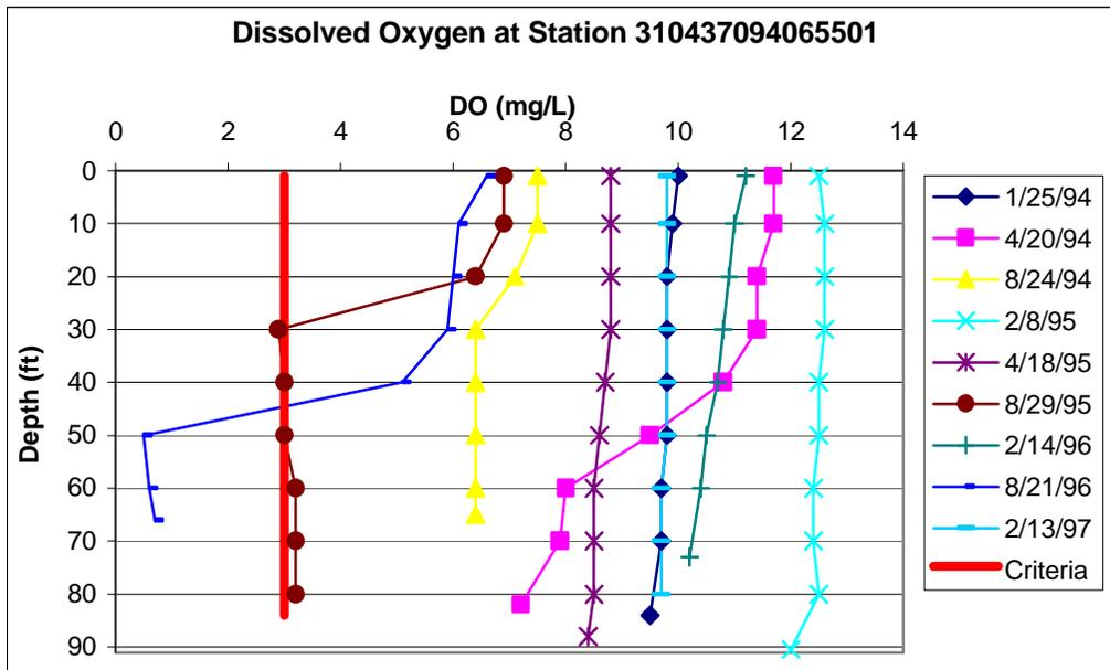
Figure 4D-11. Dissolved oxygen profile data for Sam Rayburn Reservoir at station 310437094065501 in the lower portion of the reservoir
