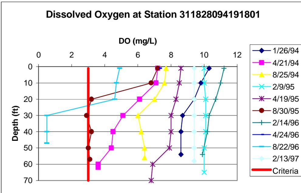
Figure 4D-5. Dissolved oxygen profile data for Sam Rayburn Reservoir at station 311828094191801 on the Attoyac Bayou arm
