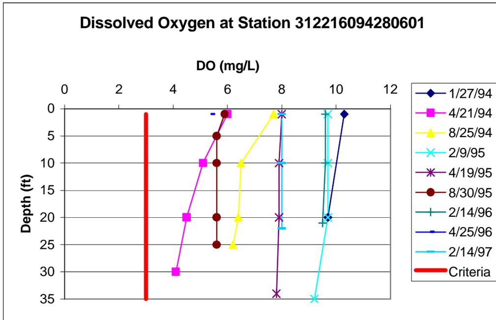
Figure 4D-3. Dissolved oxygen profile data for Sam Rayburn Reservoir at station 31221609428060 in the upper portion of the reservoir
