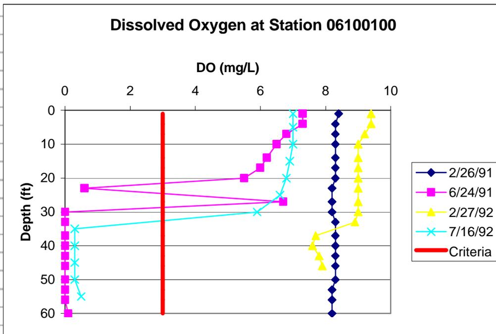
**Figure 4D-7. Dissolved oxygen profile data for Sam Rayburn Reservoir at station 06100100 in the middle portion of the reservoir**
