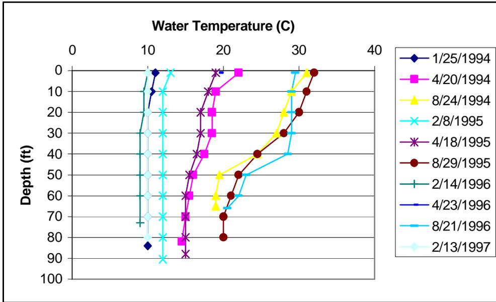
Figure 4D-10. Water temperature data for Sam Rayburn Reservoir at station 310437094065501 in the lower portion of the reservoir
