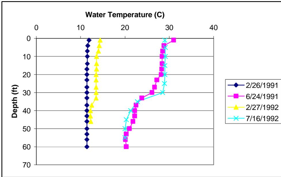
**Figure 4D-6. Water temperature profile data for Sam Rayburn Reservoir at station 06100100 in the middle portion of the reservoir**
