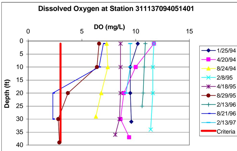
**Figure 4D-9. Dissolved oxygen profile data at Sam Rayburn Reservoir at station 311137094051401 on the Ayish Bayou arm of the reservoir**
