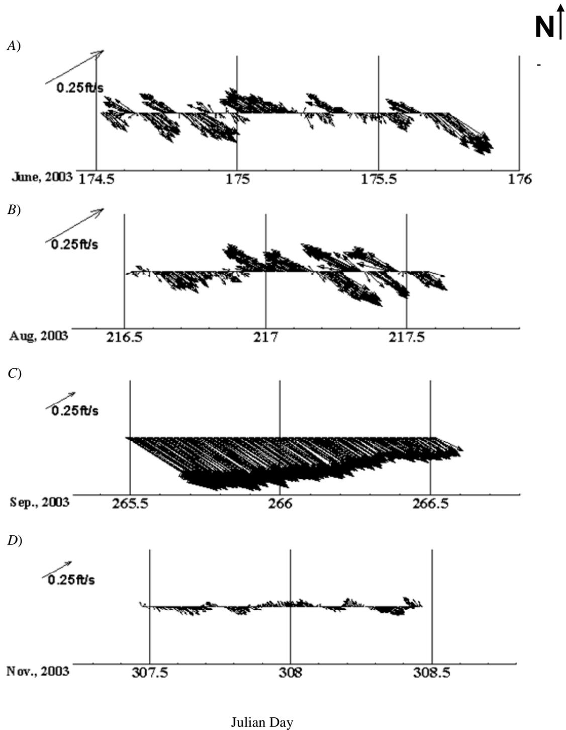
Figure 7. Total current velocities measured in the Tres Palacios River in 2003. (A) 23-25 June, (B) 4-5 August, (C) 22-23 September, and (D) 3-4 November. x-axis is Julian day with half day intervals noted by vertical gridlines. Upstream is indicated by northward pointing vectors.
