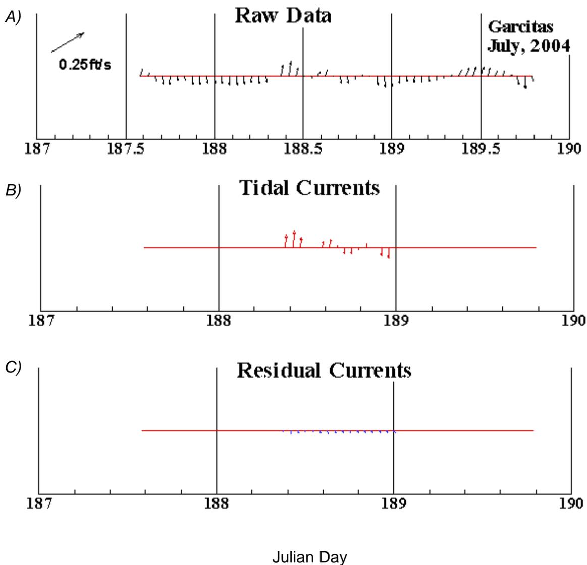
Figure 11. Flow composition at Garcitas, 6-8 July 2004. (A) Raw flow data with (B) tidal and (C) residual currents extracted. x-axis is Julian day with day intervals noted by vertical gridlines. Upstream is indicated by northward pointing vectors.
