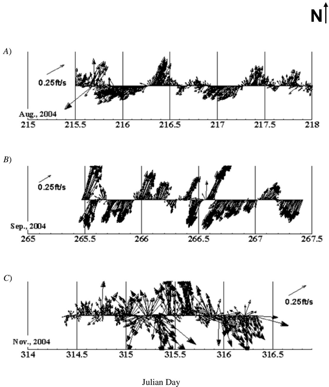
Figure 6. Total current velocities measured at Garcitas Creek in late 2004. (A) 3-5 August, (B) 22-24 September, and (C) 10-12 November. x-axis is Julian day with half day intervals noted by vertical gridlines. Upstream is indicated by northward pointing vectors.
