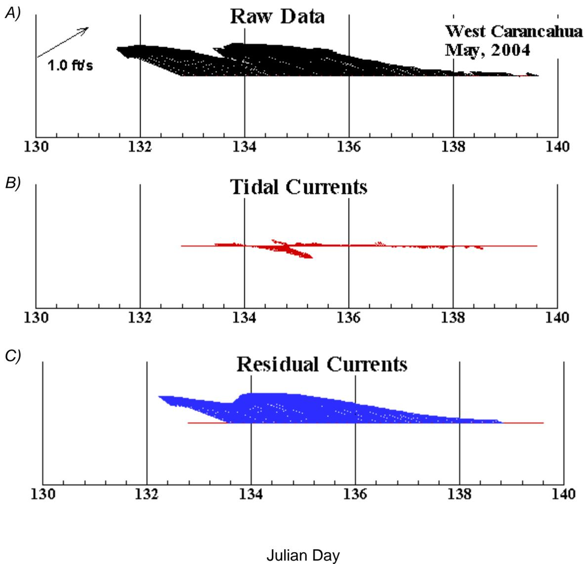
Figure 10. Flow composition at Carancahua, 12-19 May 2004. (A) Raw flow data with (B) tidal and (C) residual currents extracted. x-axis is Julian day with two-day intervals noted by vertical gridlines. Upstream is indicated by southward pointing vectors.
