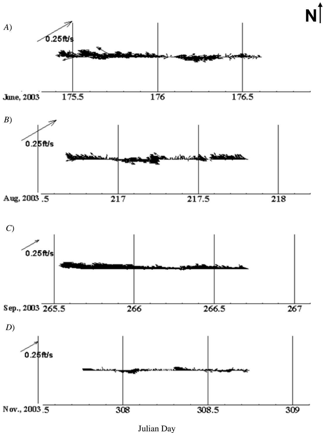
Figure 2. Total current velocities measured at West Carancahua Creek in 2003. (A) 24-25 June, (B) 4-5 August, (C) 22-23 September, and (D) 3-4 November. x-axis is Julian day with half day intervals noted by vertical gridlines. Upstream is indicated by southward pointing vectors.
