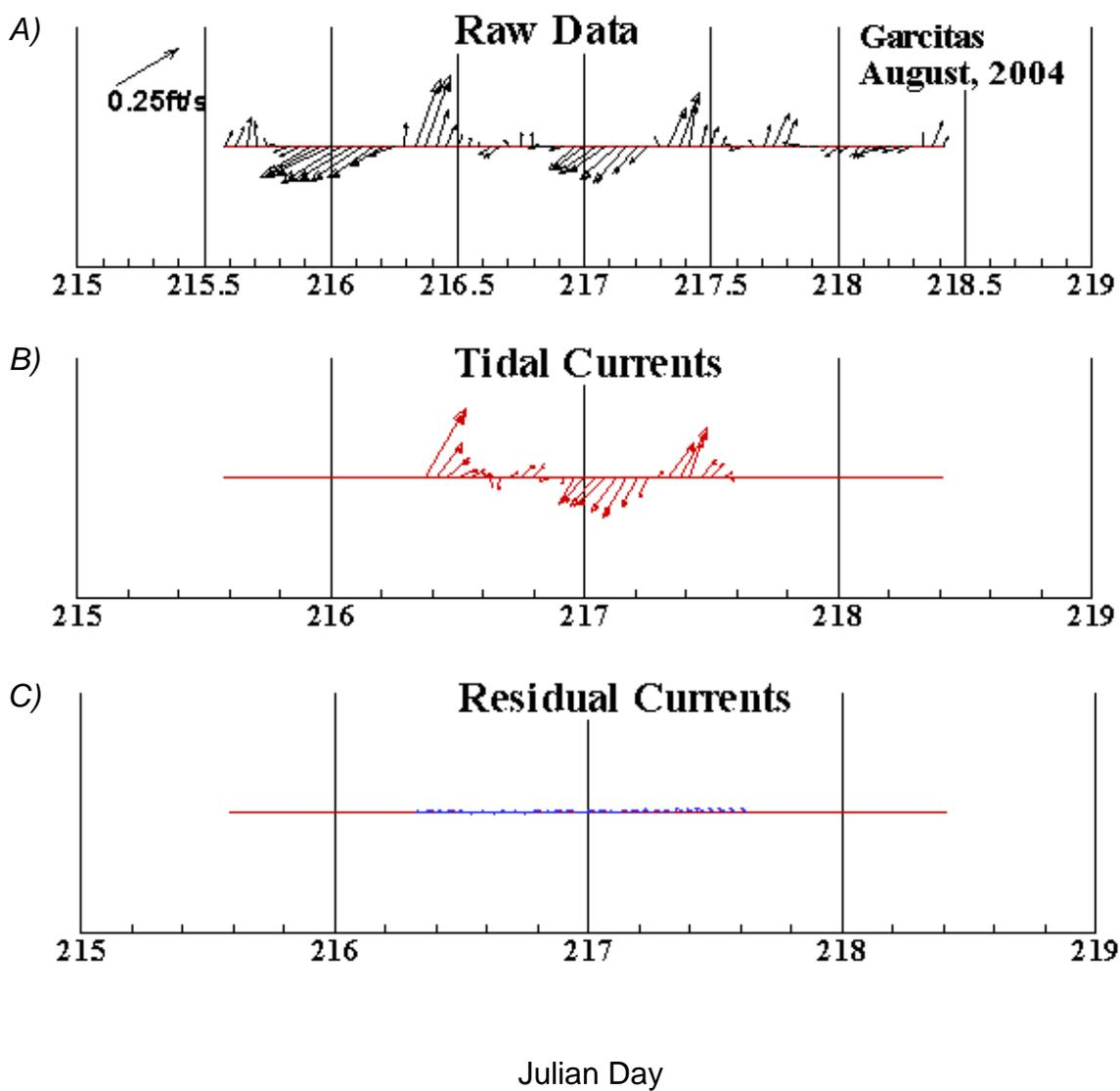
Figure 12. Flow composition at Garcitas, 3-5 August 2004. (A) Raw flow data with (B) tidal and (C) residual currents extracted. x-axis is Julian day with day intervals noted by vertical gridlines. Upstream is indicated by northward pointing vectors.
