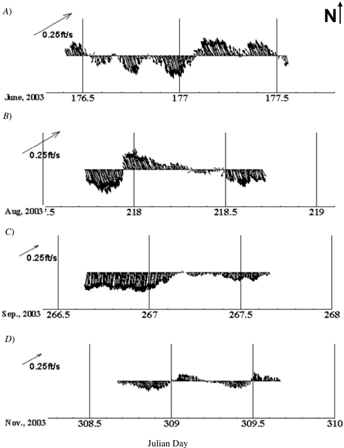
Figure 4. Total current velocities measured at Garcitas Creek in 2003. (A) 25-26 June, (B) 5-6 August, (C) 23-24 September, and (D) 4-5 November. x-axis is Julian day with half day intervals noted by vertical gridlines. Upstream is indicated by northward pointing vectors.
