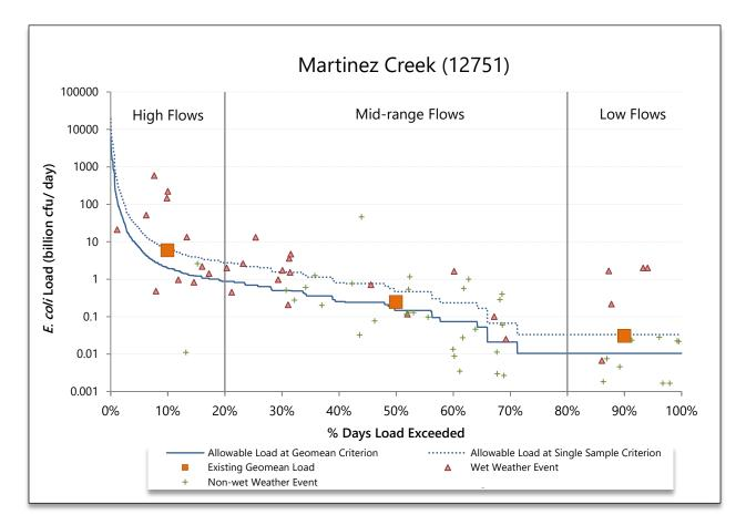
Figure 13. Load duration curve for Martinez Creek (Station 12751).
