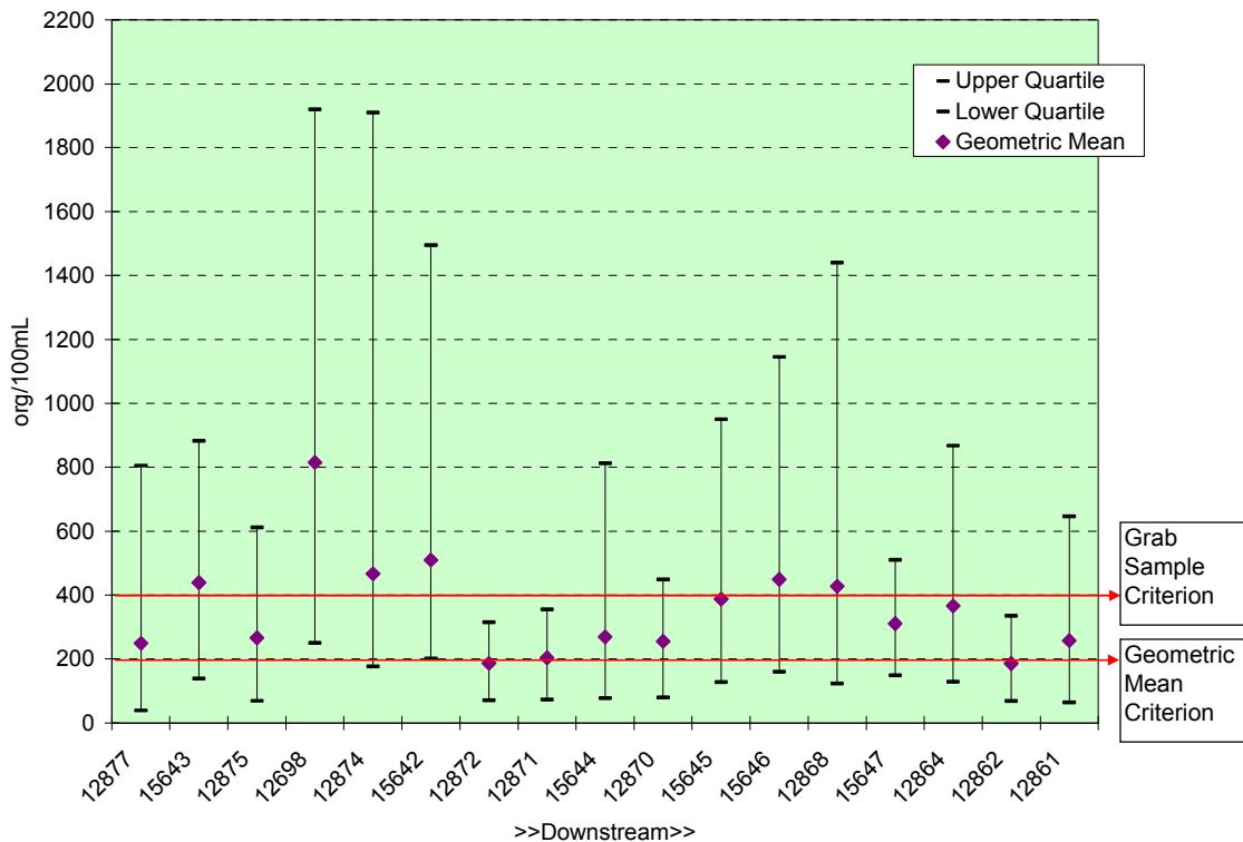
Figure 4: Fecal Coliform Sampling Results, Salado Creek
