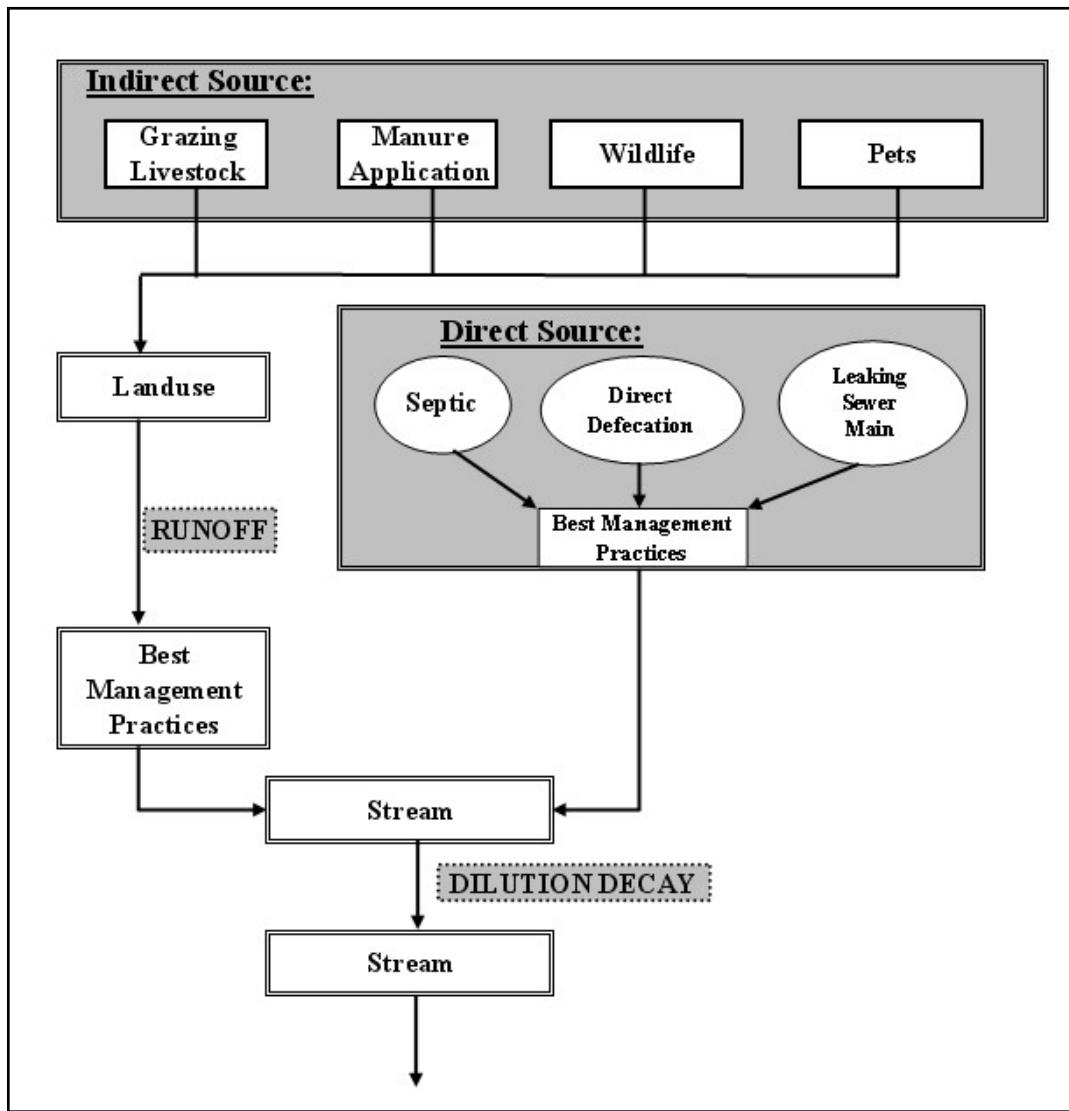
Figure 8: Methods of Nonpoint Source Loading
