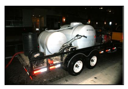
Figure 12. River Walk Implementation Plan power washer which recaptures the wastewater.
