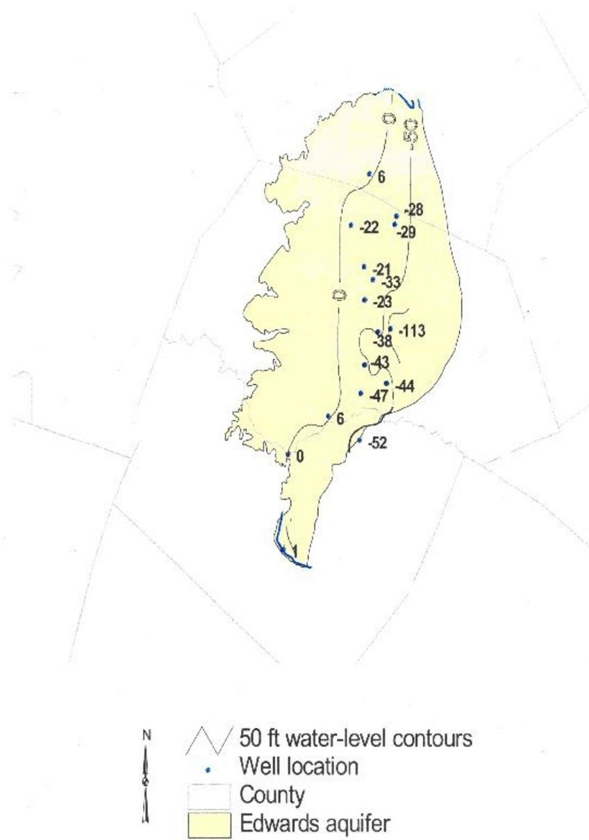
Figure 4. Water-level change in the Edwards Aquifer based on data collected 1987-1988 and data collected 1997-1998 (Ridgeway and Petrini 1999)
